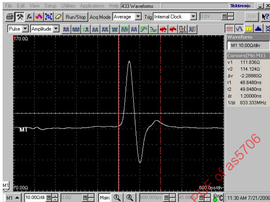
FIGURE 7 - 600 PS EXCEPTION WINDOW EXAMPLE SHOWING 1.2\text{NS}/2 = 600\text{ PS} WINDOW
